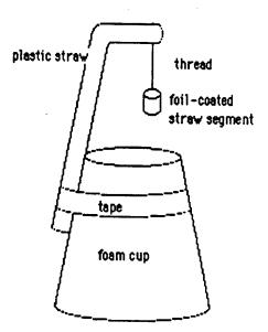
C. Set up your stand with a pith ball hanging from it on about 10 cm of thread. Rub a plastic drinking straw with wool or fur and bring it near some paper bits. Is the straw charged? Now bring the straw near the pith ball. What happens? How can you use the pith ball to test for a charged object?
