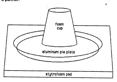
B. Rub the top surface of the foam with fur to charge it. Slowly lower the electrophorus pie plate (henceforth called the electrophorus plate) to a height of a few millimeters above the foam while holding it by the cup handle. Be careful not to touch the pie plate with your hand or arm unless instructed to do so.
