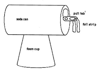
B. Take a plastic drinking straw and rub it with wool or fur. Touch the pith ball with the straw. Is the straw charged? Touch the straw to the top of the can on the electroscope. What happens to the foil leaf? How can you tell if an object is charged using the foil leaf electroscope?
