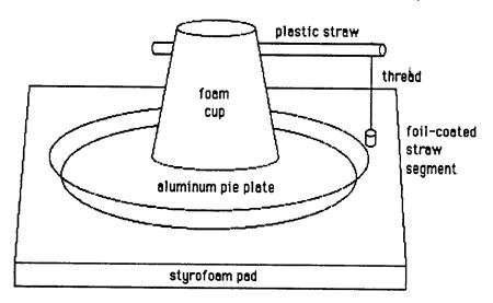
B. Now, touch the electrophorus plate briefly with your finger to discharge it, and lower the electrophorus plate onto the foam. What happens to the pith ball? Move the electrophorus plate up and down above the foam. What happens to the pith ball? What does this tell you about charges on the rim of the electrophorus plate and the pith ball as you move the electrophorus plate closer to the foam?
